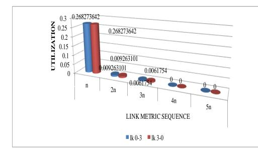
$\Box$ Whereas other links it is only when the link metric reached {4n, 5n} that the link utilization became zero.
