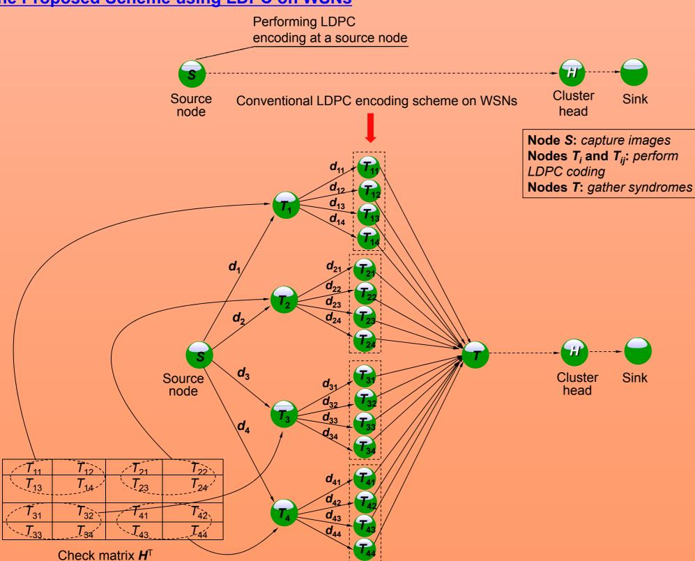
Proposed scheme for LDPC encoding on WSNs with the number of nodes  $N_n = 16$ .
