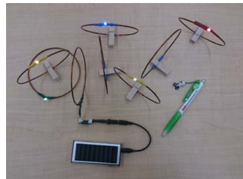
Fig. 12 Experiment of the direct-current-resonance system.
