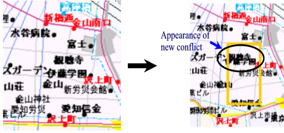
Fig 2 The context aware map synthesizer introduces new conflicts between the labels when slight scale changes are made
