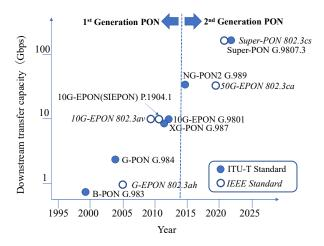
Fig. 2 Overview of standardization on PON
