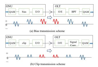
Fig. 6 Basic options on transmission schemes in SDM-PON
