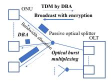
Fig. 1 System architecture of PON and its features
