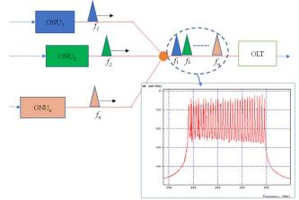
Fig. 4 Architecture of SDM-PON for upstream traffic
