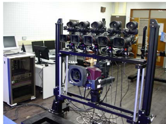
Figure 1. Hybrid camera system
