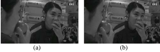
Figure 3. Re-constructed image using the SVD-based compression algorithm (a) original image (b) re-constructed image
