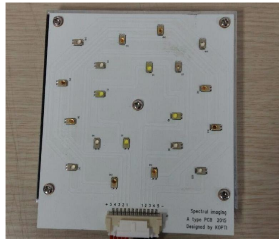
Figure 3. Illumination source consists of 20 LEDs with five kinds of color
