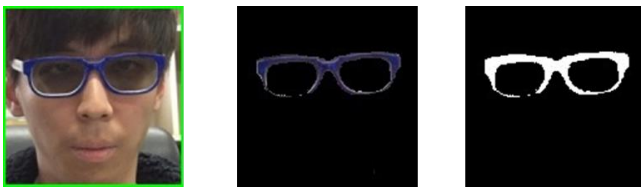
Figure 6 Transform form RGB to HSV color model
