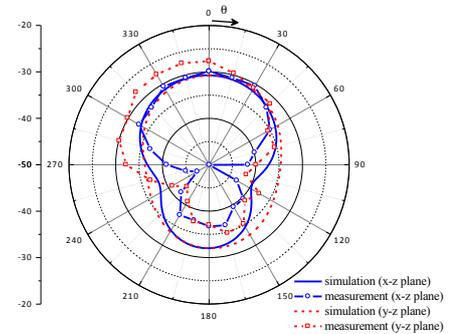
Fig. 4. Gain radiation patterns.
