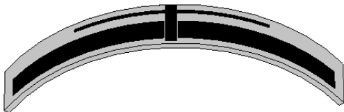
Fig. 3. Conformal antenna with a full ground plane and electromagnetically-coupled feed with stub loading.
