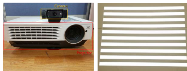
(a) Projector-camera system (b) Camera scene Figure 2. Structure of projector-camera and camera scene.
