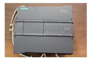
Figure 3.1 Siemens S7-1200 CPU 1214C DC/DC/Relay
