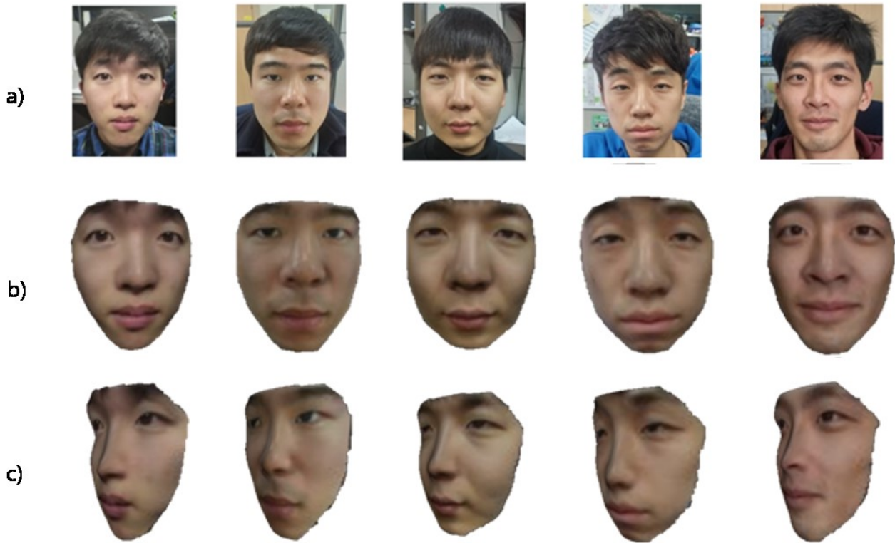
Figure 3. texture mapping on the depth map from figure 2 . First row (a) is the input image and the second row (b) shows the texture mapped 3D model by using photometric stereo from the first row's images. Lastly, the third row (c) is as well as (b) at the different angle.
