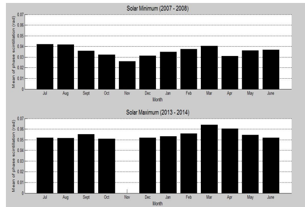
Fig. 2. Comparison of monthly mean phase scintillation \sigma_\phi at low and high solar activity periods. In November 2013, the GISTM receiver had technical problems that caused no data to be obtained for the month.
