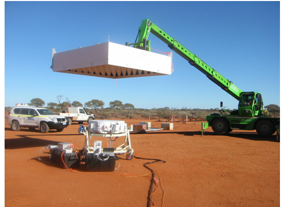
Fig. 1. Aperture-array Y-factor measurement of the Mk. II ASKAP PAF near antenna 29 at the MRO. The array is supported on the ground so that it points face-up at the zenith. A telehandler is used to position a large microwave absorber load over and alternately away from the array.
