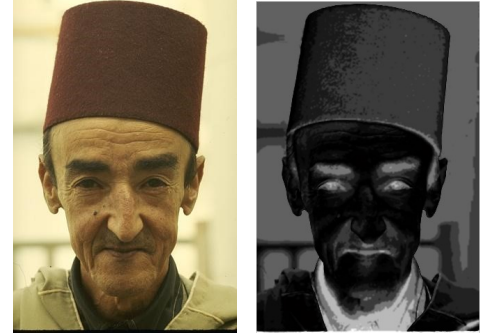
(a) Zoom-in image (b) Depth map of (a) using saliency-based depth estimation [1]
