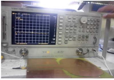
Fig. 2 Measurement of reflection coefficient using network analyser
