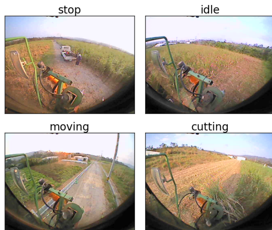
Figure 2. Four working states of the harvester
