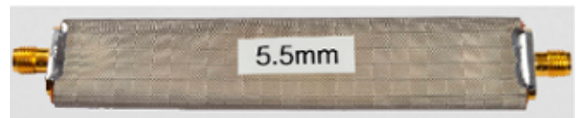
Fig. 1. Flexible shielded stripline fabricated using “Shieldit Super” and fleece.
