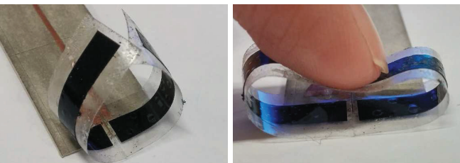
Fig. 3. PEDOT antenna in two bending configurations.
