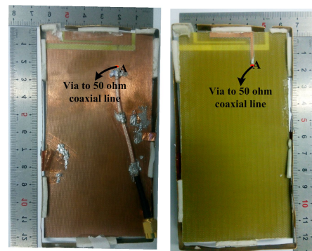
Fig.6 Photos of the manufactured slot antenna for for WWAN Metal-Rimmed smartphone applications: (a) Front side, (b) Back side
