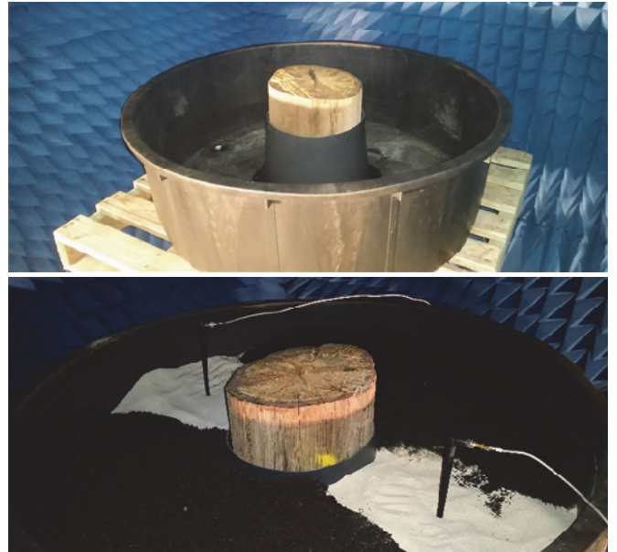
Fig. 2. Before and after shots of a 300mm deep by 1m diameter annulus filled with soil and sand, surrounding a rotating pole sample. 6dB (ground-penetrating) wideband whip antennas are shown in transmission-mode.
