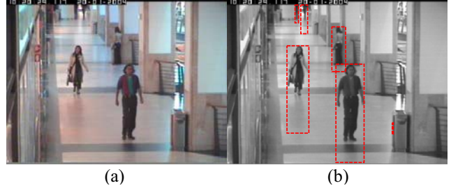
Fig. 1. Foreground extraction. (a) Input image (CAVIAR data set, 384 \times 288 ). (b) Detected foreground
