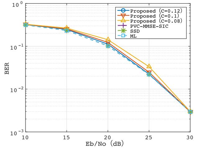
Fig. 4. BER performance ( $n = 4, m = 2$ , 16-QAM)
