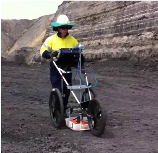
Fig 4. Deployment of commercial cart-mounted GPR antenna and controller system at an open-cut coal mining operation.
