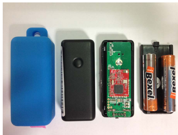
FIGURE 1: A REDBEAR iBEACON NODE WITH 2 AAA BATTERIES
