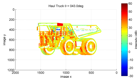
Fig. 5: Simulated response at ( 43^\circ ). Note the significant return from the lip of the bucket.
