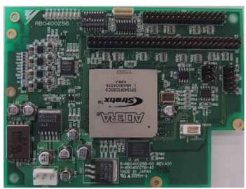
Fig4. A magnetic encoder evaluation board
