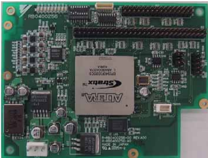
Fig4. A magnetic encoder evaluation board
