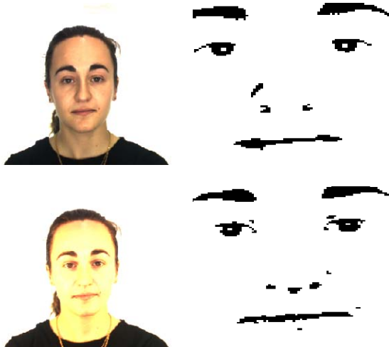
Figure 4. Binarization result. Original images under different illumination conditions (left column), corresponding binarized images (right column).
