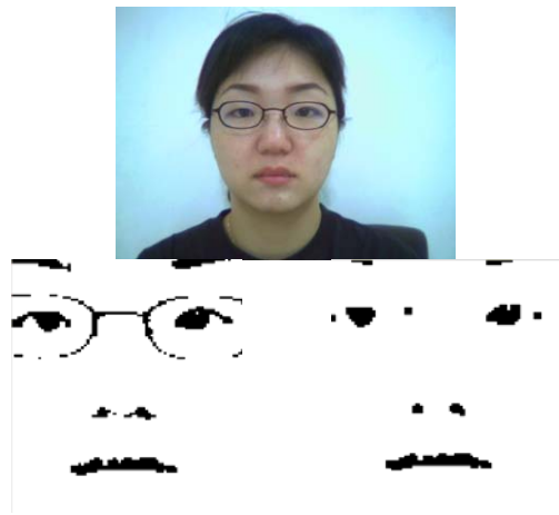
Figure 5. The result of morphology: original image (top row), binarized image (bottom left), and morphologied image (bottom right).
