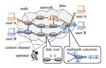
Fig. 1. System configuration
