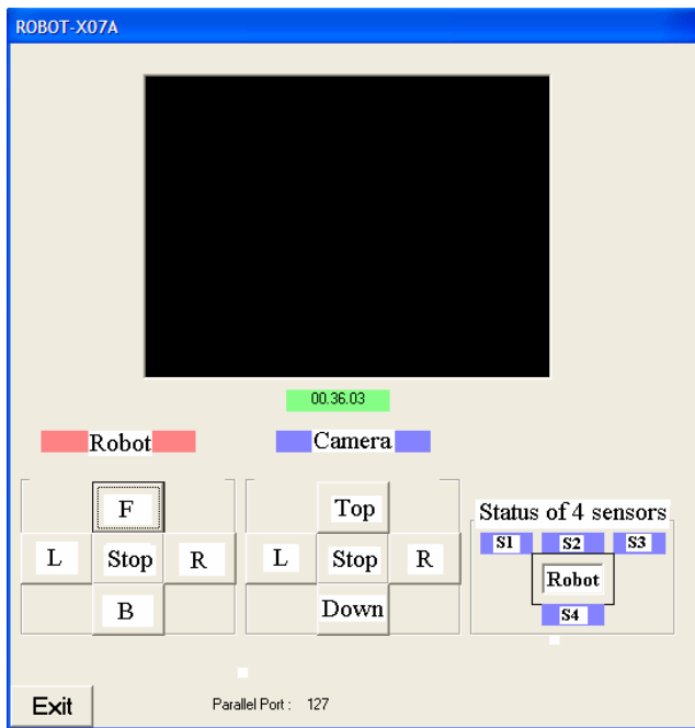
Figure 4 Graphic user interface (GUI) for communication between the computer/notebook and robot.
