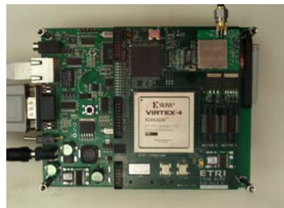
Figure 7. Test board for AT-DMB receiver system
