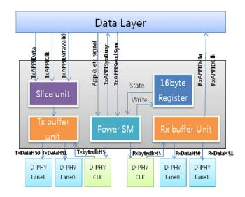
Figure . Overall block diagram of PHY adapter
