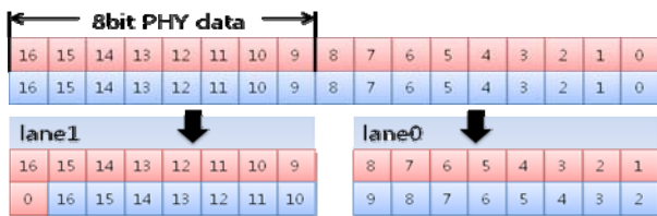
Figure 4. Transmission of 17-bit of symbols with two lanes
