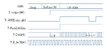
Figure . Transmisson of packets at ON mode
