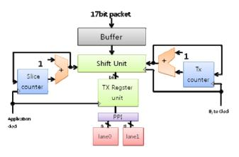
Figure . Schematic of Tx buffer
