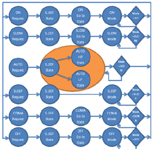
Figure 7. State transitions of power management state machine
