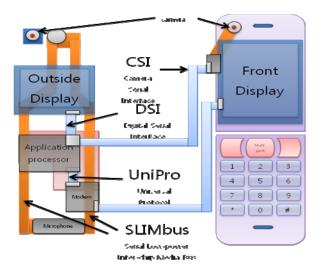
Figure . MIPI interfaces for mobile application
