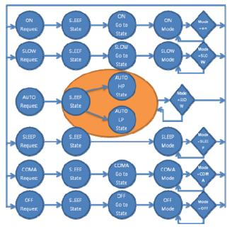
Figure . State transitions of power management state machine
