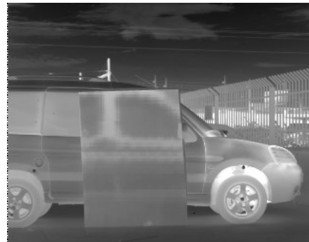
Fig. 1: Fusion of an IR and a sub-mm wave image of a car behind a wooden panel.
