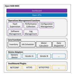
Fig. 3. System Architecture of Open RAN NMS
