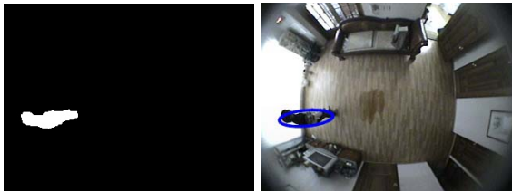
Figure 4. (a) After removing noise from the image in Figure 3(b); (b) The result of elliptical mapping
