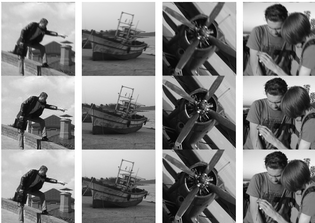
Figure5: The results of the ringing artefact removing algorithm. First row: The blurred images with varying blur direction and estimated PSF distance from 10 to 15 pixels. Second row: The results produced by deblurring algorithm. Bottom row: The results produced by deringing algorithm
