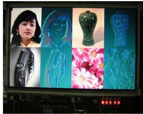
Figure 7. Original and filtered images on a display device of a prototyping board
