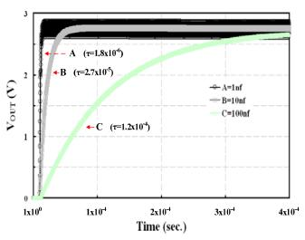
Fig. 5. Transient response of output voltage with variation of capacitance in the LP filter
