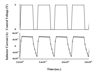
Fig. 4. Inductor current with on-off switching time.
