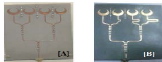
Fig. 2. Fabricated array with maximum radiation at 0^\circ and 45^\circ respectively
