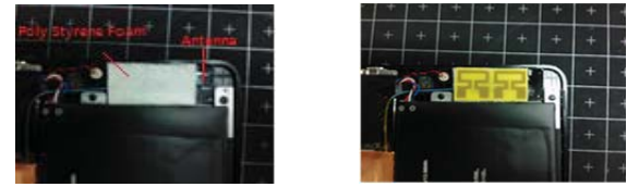
Fig. 4. (a) Table PC without EBG. (b) Table PC with EBG.
