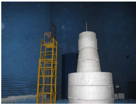
Fig.3 a dipole antenna test in anechoic chamber
