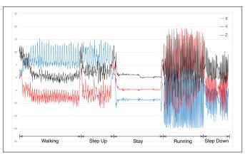
Fig. 1. Different patterns of accelerometer sensor according to user behaviors
