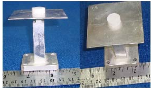
Fig. 4. Photograph of the fabricated antenna
