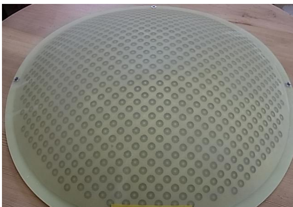
Fig. 3. A photograph of the fabricated FSS-embedded radome that was used for the measurement.
