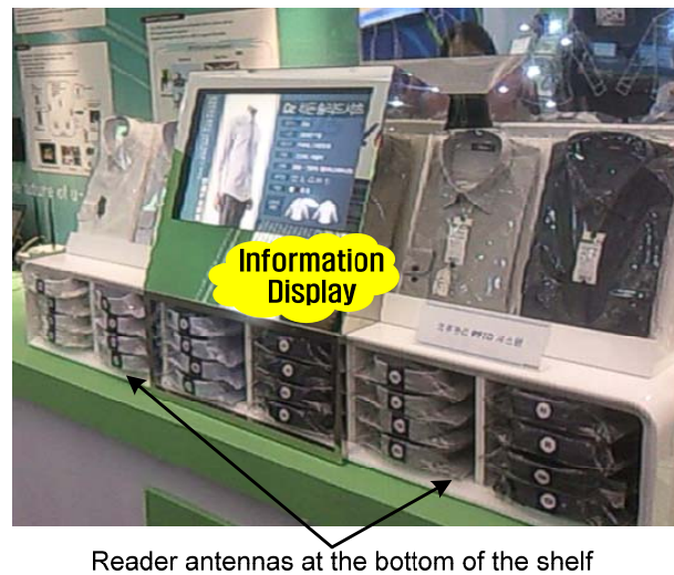
Figure 4: Designed RFID shelf configuration in apparel
