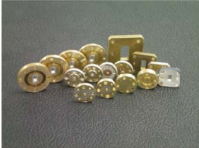
Figure 3. Waveguide shims that are to be loaded with material samples.
