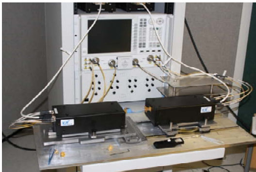
Figure 7. The rail system constrains the movement of the extension heads and cables.
