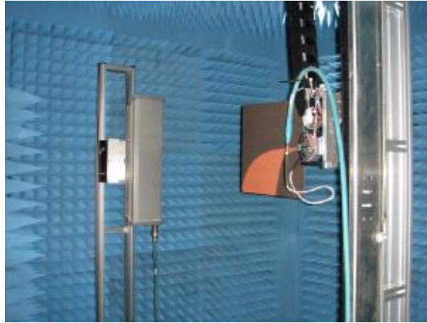
Figure 2: Photograph of experiment in the anechoic chamber.
