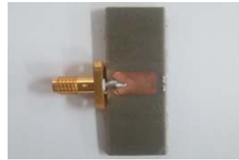
(b) ENG ZOR antenna at 14 GHz
